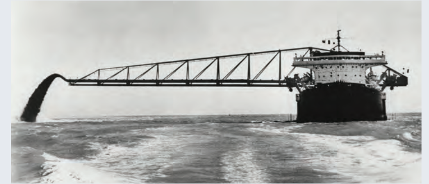
The Zulia , a large and highly effective side-casting boom and hopper dredge, was conceived, designed and built by Ludwig. Created to deepen the entrance to Lake Maracaibo in Venezuela to open access to massive oil tankers, it removed more "spoil" in 10 days than small hopper dredges had removed in two years.
